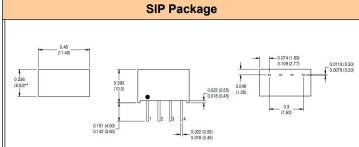
All dimensions in inches  $\pm 0.01$ (mm $\pm 0.25$ mm). All pins on a 0.1(2.54) pitch and within  $\pm 0.01(0.25)$ of true position. Weight: 1.48g (DIP)1.30g (SIP)
