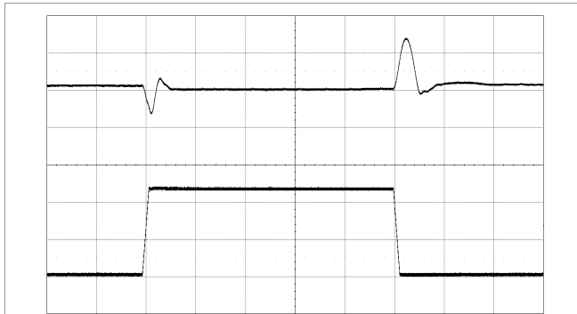
Output voltage response to load current Step-change (12.5-37.5-12.5 A) at: T_{P1} = +25\text{ }^\circ\text{C} , V_I = 12\text{ V} , V_O = 1.0\text{ V} di/dt = 2\text{ A}/\mu\text{s} , f_{sw} = 320\text{ kHz} C_O = 470\text{ }\mu\text{F}/10\text{ m}\Omega Top trace: output voltage (200 mV/div.). Bottom trace: load current (10 A/div.). Time scale: (0.1 ms/div.).
