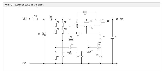
This circuit has been evaluated successfully over temperature for nominal 110 VDC input worst case 3.5 Vnom surge as specified in RIA12. Waveforms obtained are shown in Figures 3. Suggested component values for 110V input are given in Table 4.
