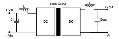
If it is required to decrease the input/output ripple an "LC" filter network can be installed on the input and output of the converter (see above).
