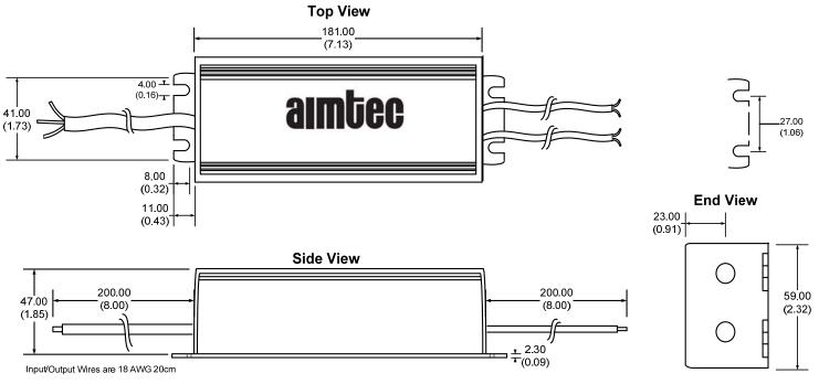
Measurements in Millimeters (inch) Case Tolerance: ±0.5 (±0.02)
